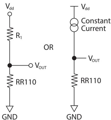
**RR110 Magnetoresistance Application Circuit**
